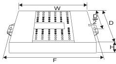
Height = 50mm (108mm including plug and lead) Width = 315mm (361mm including mounting feet) Depth = 205mm Fixing Centres = 340mm Weight = 1.85kg
