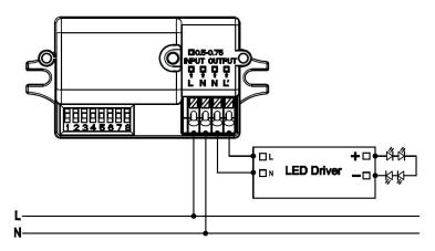
\*The sensor is designed for connect one load only. Connect more than one loads may damage the sensor.
