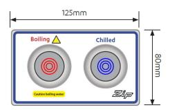
Cut the hole for the sensor control panel using the diagram below, the dimensions are symmetrical.
