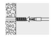
Place Screw in Plug & tighten until secure
