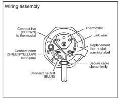
NOTE: BEAB approval only applies when the components are assembled correctly as shown in the diagrams above.
